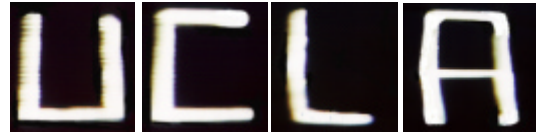
Figure 9 : Four characters (UCLA) displayed individually by the laser scanning system shown in Figure 8.
